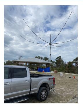
5 band hex beam on N4LJT truck bumper mount and push up pole
