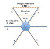
Perhaps the easiest part of the project was fabricating the spreader cords. 7 cords 128 inches long (including the "s" hooks on each end) and one shorter cord, about 90 inches. I pre-streched the dacron cord when I made the measurements to cut.
