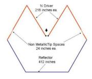
Next, I assembled the antenna wire sets. So far I have only built the 20, 15, and 10 meter sets. Included on the web site is a chart that gives the dimensions for the directors, reflector, and spacers. The 20 meter 16 AWG <u>pvc</u> covered braided wire sketch is shown. The wire cost me 27 cents a foot. About \$77 for all the wire needed for the 6 bands.
