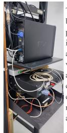
The picture on the left shows the back view of the rack mounted repeater system. On the bottom shelf is the power supply for the 100 watt amplifier. Above that is the back view of the repeater/controller, and above that is the computer used to control and adjust the repeater/controller settings. Several items remain to be done. to "clean up" and standardize the installation.
