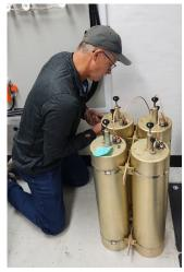
The repeater was removed from service at about 9:30 am that morning. In the photo at the left, KM4GX is in the final stages of preparing the RF cavities for their trip to the tuning bench.. As you can see, there are 4 tuned cavities. The two on the left (top and bottom) are hooked in series and connect the repeater receiver section to the
