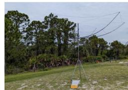
Hex beam set up on 20, 15, 12, and 10 meters
