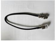
Pigtail and adapter for ICOM NXDN HT's. Used to connect to an external antenna. Contact Bernie Schmelz if you would like one. Provided at cost for CCFLARES/EARS members.
